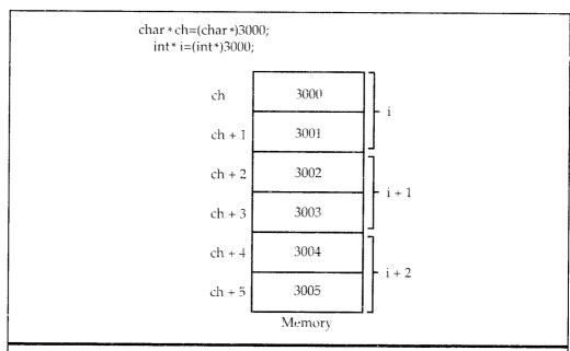
**Figure 5-2.** All pointer arithmetic is relative to its base type (assume 2-byte integers)
