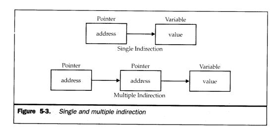
A variable that is a pointer to a pointer must be declared as such. You do this by placing an additional asterisk in front of the variable name. For example, the following declaration tells the compiler that **newbalance** is a pointer to a pointer of type **float**:
